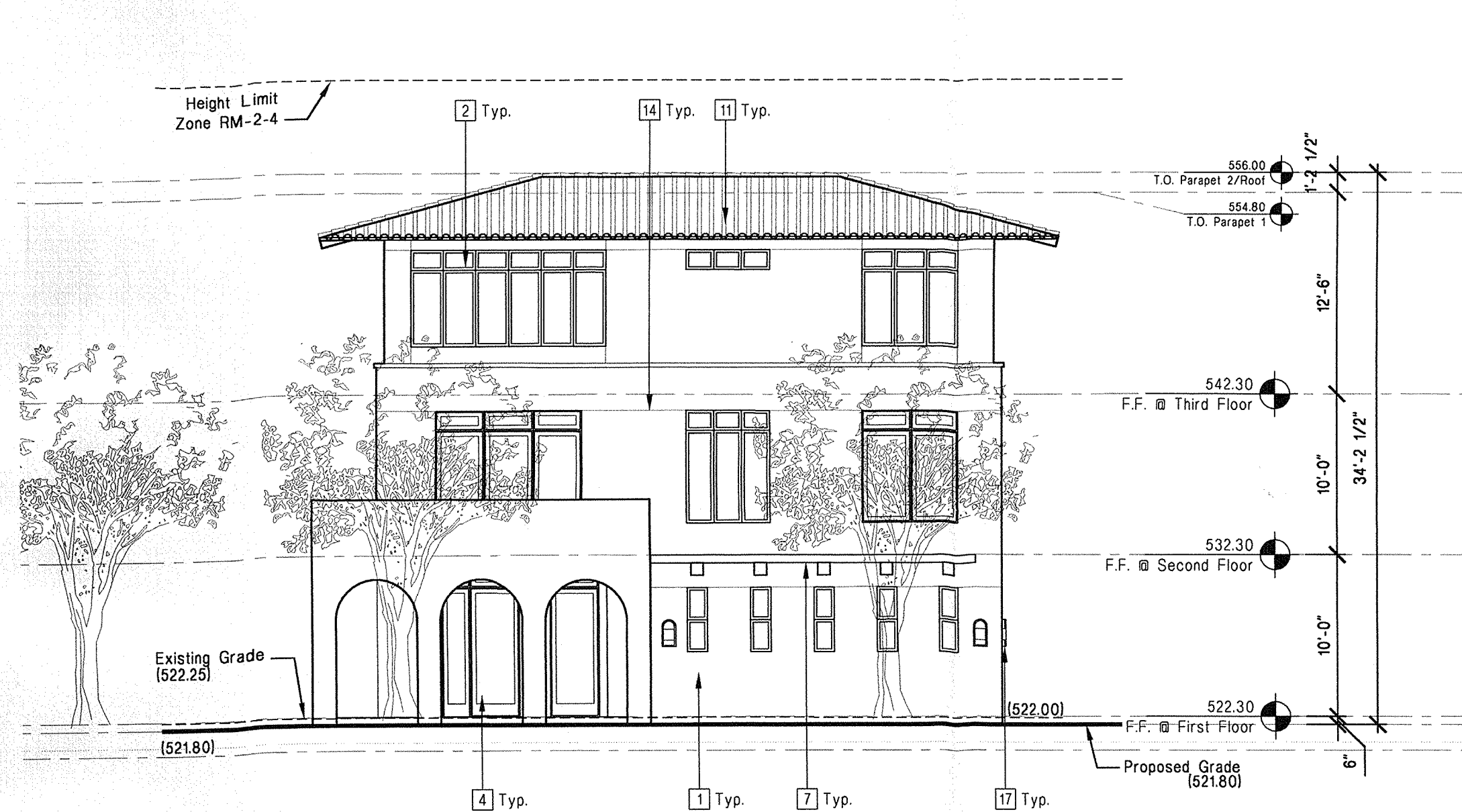
8 Building 'A3.1' East Elevation scale: 1/8" = 1'-0"
