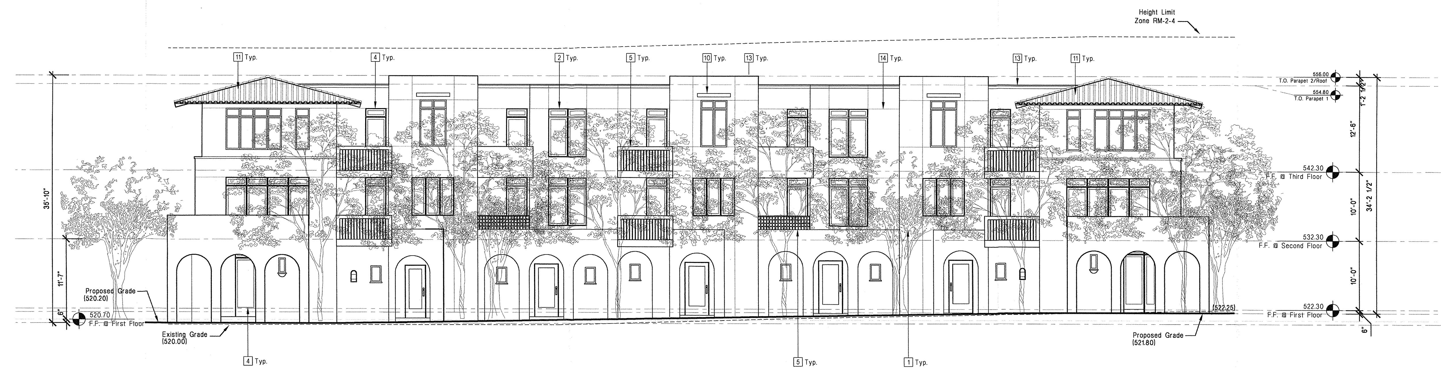
4 Building 'A3.1' South Elevation scale: 1/8" = 1'-0"
