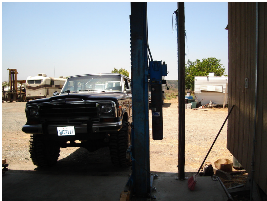
Photograph #27 View of hydraulic reservoir associated with automobile lift in automobile maintenance area at Tommy Tucker Automobile Storage/Sales.
