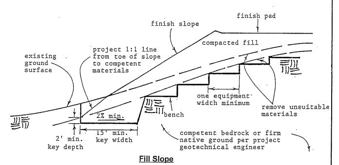
Note: Key and benching details shown herein are subject to revisions by the project geotechnical engineer based upon actual site conditions. Back drains may also be necessary as determined by the project geotechnical consultant.
