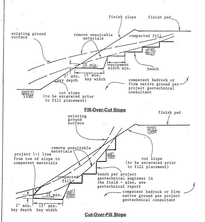
Note: Key and benching details shown herein are subject to revision by the project geotechnical engineer based upon actual site conditions. Back drains may also be necessary as determined by the project geotechnical consultant.
